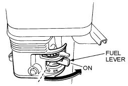
Figure 6. Engine Fuel Valve Lever (ON Position)
